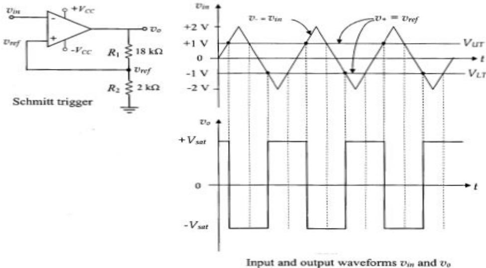
Input and output waveforms  $v_{in}$  and  $v_o$
